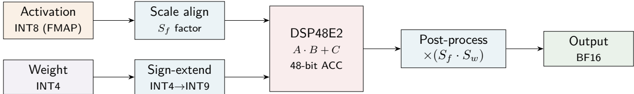
Figure 3.1: DSP48E2 datapath (W4A8). INT8 activations are sign-extended to INT9; INT4 weights are sign-extended to INT4. The 9 \times 4 b product accumulates in a 48-bit DSP48E2 register; the joint BF16 scale factor S_f \cdot S_w is applied once in the Post-process stage.
